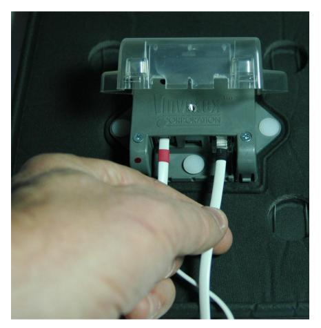
3. If another Halotile will be attached to this Halopod, plug in the BLACK marked connector of a new white cable into the right connector of the HaloPod.
