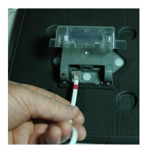
2. Raise the Splash Cover on the HaloPod and plug in the RED marked connector on the white cable from the previous HaloTile or from the IMS controller if the first tile, into the left connecter on the Halopod, marked by the red dot.
