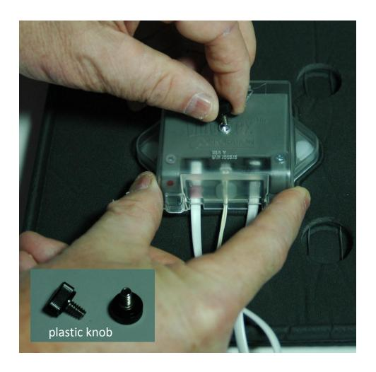
5. Hold down the Halopod splash cover (making sure the cables are in the slots provided for them) and insert the plastic knob retaining screw into the splash cover as shown.
