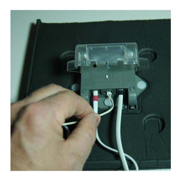
4. If the ceiling clip will be used, connect it to the center connector of the HaloPod and push in gently.
