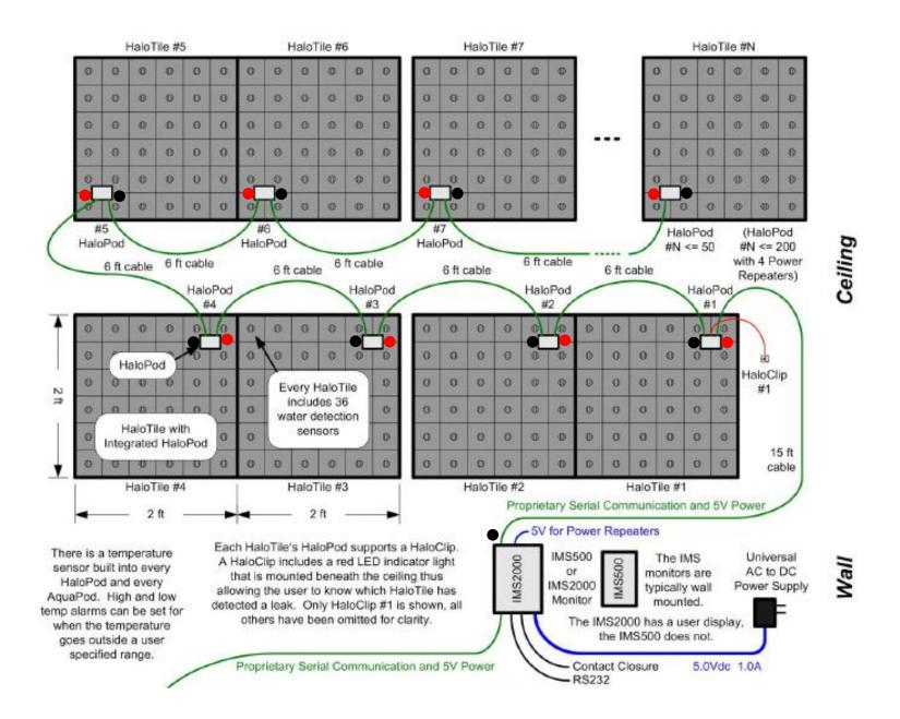
HaloTile Installation Block Diagram
